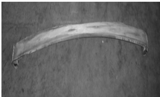
Fig. 3. Complete composite mono leaf spring
