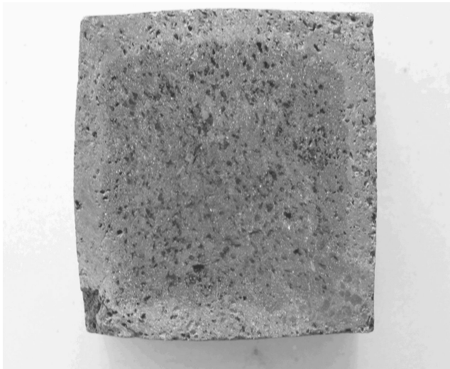
Fig. 8. Picture of the sample with 5 % rubber waste after burning at the highest 950 °C temperature ( \times 1 times)
