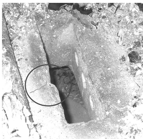
Fig. 1. Examples of castable products destruction in boiler (size (40 \times 20 \times 5) \text{ cm} and (60 \times 40 \times 10) \text{ cm} )
