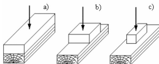
Fig. 1. Cases of wood compressing perpendicular to grain [6]
