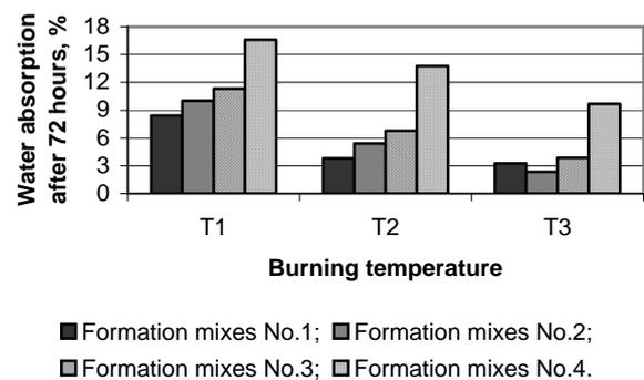
**Fig. 6.** Dependence of water absorption after 72 hours on the burning temperature
