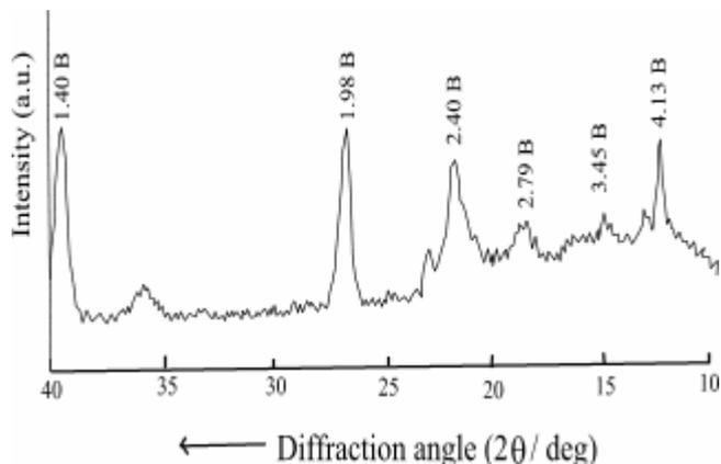
**Fig. 2.** X-ray diffraction pattern of the waste catalyst at burning temperature 1000 °C (notation index is presented in the text)
