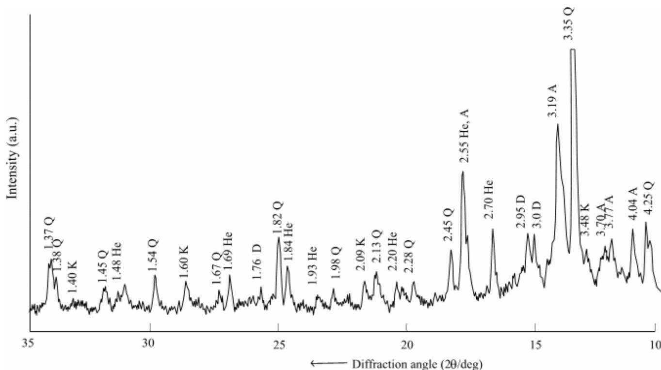
**Fig. 10.** X-ray diffraction pattern of examples of the ceramics body with 5 % of catalyst additives at burning temperature 1100 °C (notation index is presented in the text)
