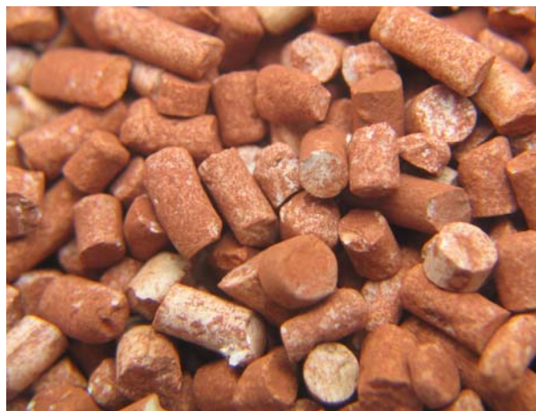
Fig. 1. Picture of the catalyst previously been in service
