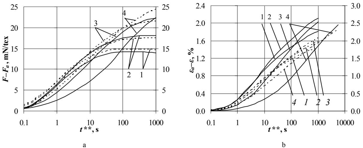
**Fig. 6.** Inverse stress relaxation (a) and viscoelastic recovery (b) curves of CA yarn in R- (—, left scale) and C- (----, right scale) test cycles, mode II ( $F_c = 71.5$  mN/tex);  $\theta_i$ : 1 – 1 s, 2 – 10 s, 3 – 100 s, 4 – 1000 s
