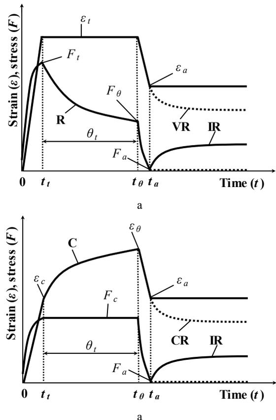
Fig. 1. The testing cycles: a – test at constant elongation; b – test at constant force
