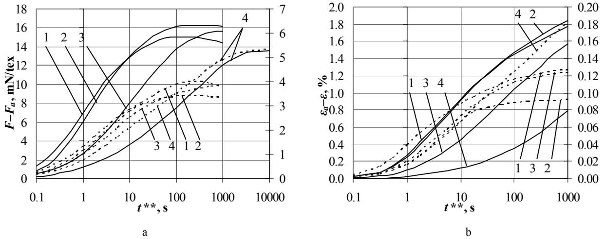
**Fig. 4.** Inverse stress relaxation (a) and viscoelastic recovery (b) curves of CA yarn in R- (—, left scale) and C- (----, right scale) test cycles, mode I ( $\epsilon_i = 9.1\%$ );  $\theta_i$ : 1 – 1 s, 2 – 10 s, 3 – 100 s, 4 – 1000 s
