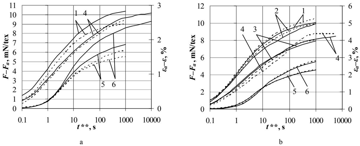
**Fig. 5.** Inverse stress relaxation (IR, left scale) and viscoelastic recovery (VR (CR), right scale) curves of PES yarn in R- (—) and C- (----) test cycles. a – mode I, ( $\epsilon_i = 14.4\%$ ); b – mode II, ( $F_c = 319.6$  mN/tex); IR curves as  $\theta_i$ : 1 – 1 s, 2 – 10 s, 3 – 100 s, 4 – 1000 s; VR and CR curves as  $\theta_i$ : 5 – 1 s, 6 – 1000 s
