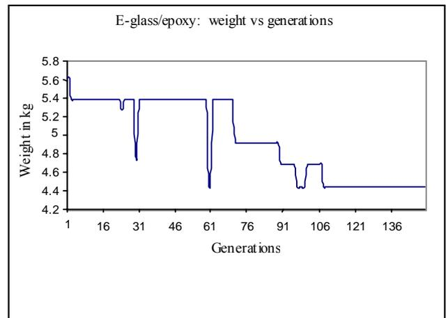
**Fig. 3.** Variation of weight of E-glass/epoxy drive shaft with number of generations
