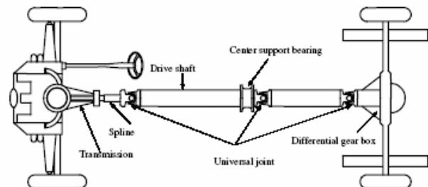
**Fig. 1.** Conventional two-piece drive shaft arrangement for rear wheel vehicle driving system
