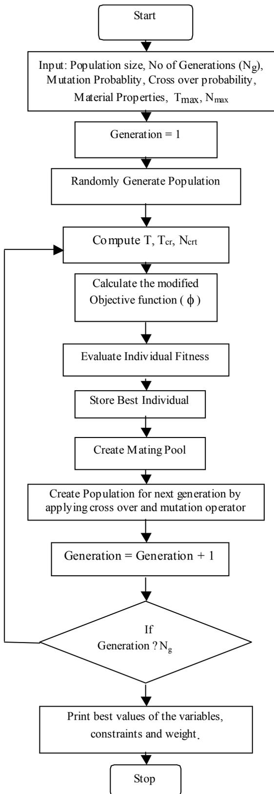
Fig. 4. Flow chart of GA based optimal design
