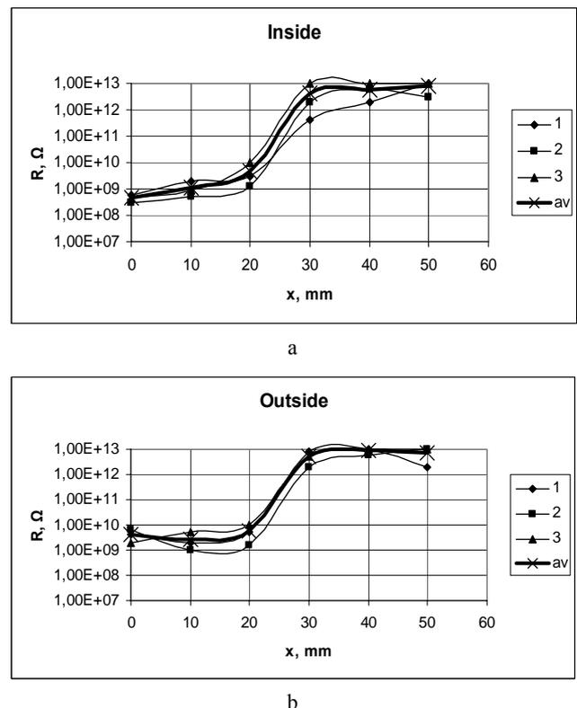
**Fig. 7.** Antistatic layer resistance along EOS cylinder: a – inside the cylinder, b – outside the cylinder. The curves 1, 2, 3 present resistance of the layer, measured turning the cylinder around its axis every 120° and the “av” presents average value of layer resistance
