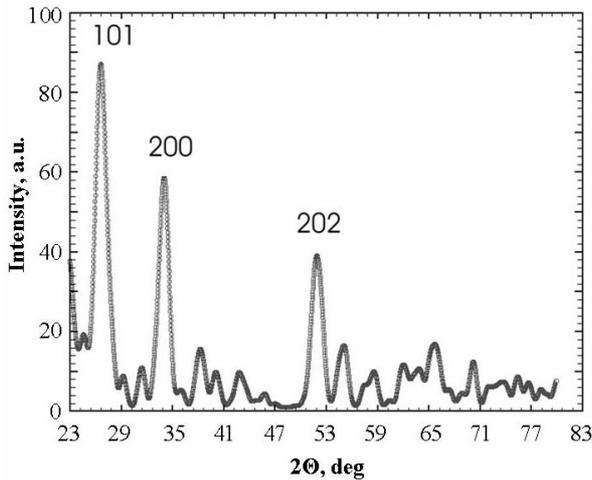
Fig. 8. XRD pattern of the SnO<sub>2</sub> antistatic layer ( $d = 100$  nm)
