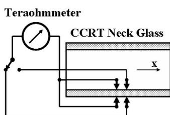
Fig. 3. The schematic of resistance measurement
