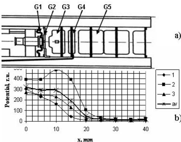
**Fig. 6.** Schematic of electron gun electrodes (a) within a CCRT tube and corresponding potential changes on the external side of the cylinder along the axis (b): 1 – 20 min. after switching on the CCRT, 2 – 40 min., 3 – 80 min., where G1-G5 are the electrodes of EOS
