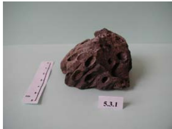
Fig. 8. Microstructure of blast furnace slag, partly crystallized
