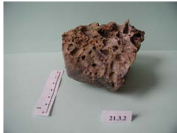
Fig. 7. Microstructure of blast furnace slag, glassy structure
