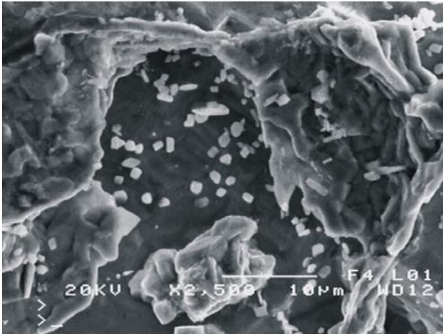
Fig. 6. SEM photographs of the sample after selective dissolution; electrolyte No. 1 b
