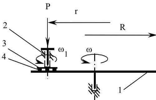
**Fig. 2.** Scheme of experimental device for studying resistance of graphic element print to mechanical impact (friction): 1 – disc; 2 – holder; 3 – specimen disc; 4 – specimens;  $P$  – load;  $\omega$ ,  $\omega_1$  – angular velocities of the disc and specimen disc, respectively
