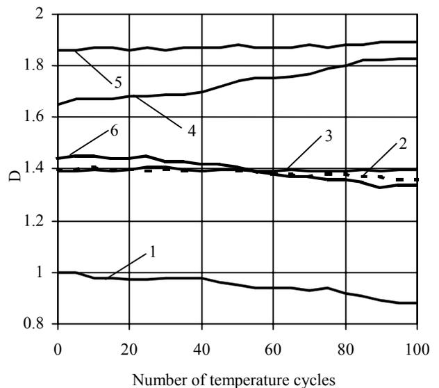
**Fig. 4.** BC optical density dependence upon the number of temperature cycles. Printed with ultraviolet inks: 1 – Vellum paper, 2 – Thermal Top paper, 3 – Pharma Matt paper, 4 – Rafla Coat paper, 5 – Rafla Coat paper (340 lpc liniature raster roller was used for printing), 6 – PP White film
