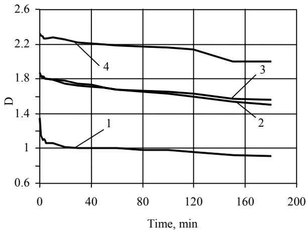
**Fig. 5** Dependence of BC optical density upon the duration of mechanical impact (friction) after temperature change:  $v_1 = 0.47$  m/s,  $P = 441.45 \times 10^{-3}$  N/cm<sup>2</sup>. Printed with water-base ink: 1 – Vellum paper, 2 – Thermal Top paper, 3 – Pharma Matt paper, 4 – Rafla Coat paper
