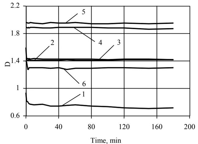
**Fig. 6.** Dependence of BC optical density upon the duration of mechanical impact (friction) after temperature change:  $v_1 = 0.47$  m/s,  $P = 441.45 \times 10^{-3}$  N/cm<sup>2</sup>. Printed with ultraviolet inks: 1 – Vellum paper, 2 – Thermal Top paper, 3 – Pharma Matt paper, 4 – Rafla Coat paper, 5 – Rafla Coat paper (for printing 340 lpc liniature raster roller was used.), 6 – PP White film
