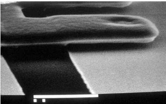
**Fig. 5.** Contact tip gap. Mark size 10  $\mu\text{m}$
