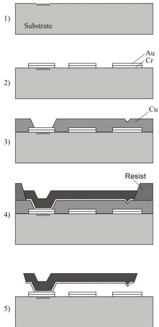
**Fig. 2.** Fabrication sequence of a microelectromechanical switch: 1 – patterning and etching of the microstructures in the source support area, 2 – “lift-off” photolithography of Cr-Au bilayer, 3 – processing of a sacrificial Cu layer, 4 – evaporation and “lift-off” of Au layer; patterning of the thick resist and Ni electroplating, 5 – removal of a sacrificial layer
