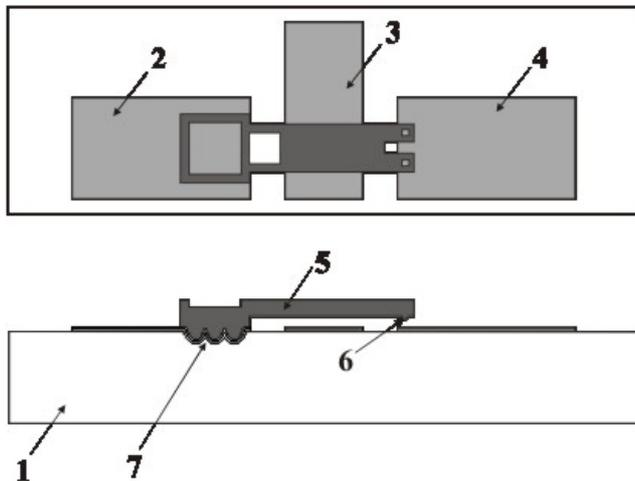
**Fig. 1.** Schematic illustration of the fabricated microelectromechanical switch: 1 – substrate, 2 – source, 3 – gate, 4 – drain, 5 – cantilever beam, 6 – contact tip, 7 – microstructures (support area)
