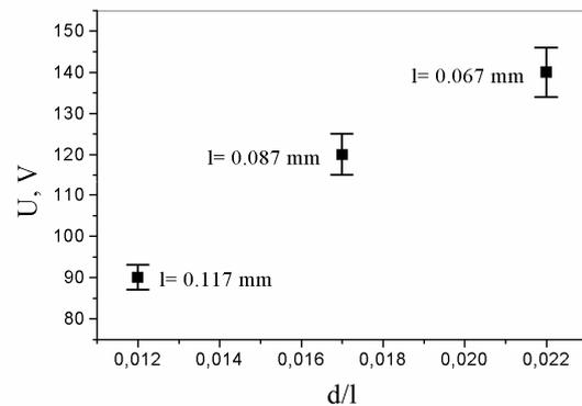
**Fig. 8.** Actuation voltage versus relation of a gap space ( $d$ ) and cantilever beam length ( $l$ ). The thickness of the cantilever beam is about 1.5  $\mu\text{m}$
