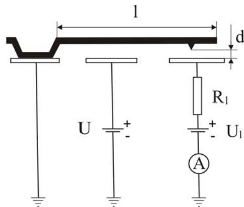
**Fig. 7.** A measurement circuit of a microelectromechanical switch,  $l$  – length of the cantilever,  $d$  – contact tip gap
