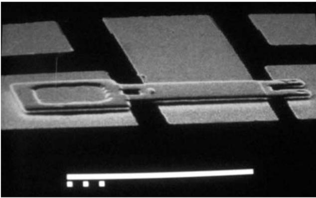
**Fig. 3.** Top view of a microelectromechanical switch. Mark size 100  $\mu\text{m}$
