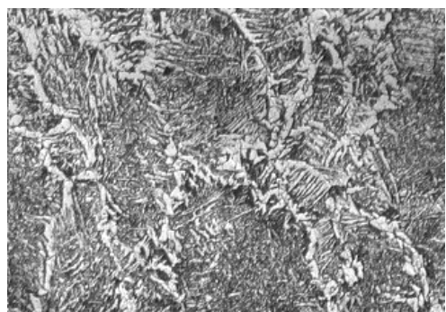
Fig. 5. Microstructure of layer of A2 alloy (×150)
