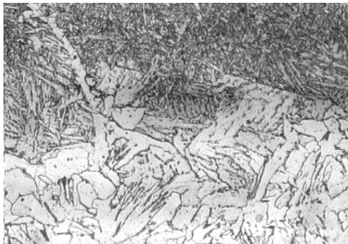
Fig. 6. Microstructure of fusion zone of B2 alloy (x150)
