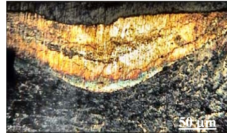
Fig. 2. Segment of brass coating on the friction surface (cross section)
