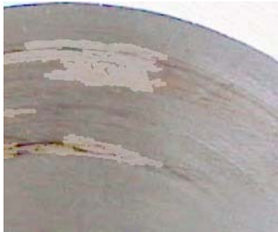
Fig. 4. Disk surface after the friction test with 50/50 block: light segments – copper coating (2:1)
