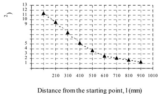
**Fig. 2.** The distribution of the density of heat flux, subject to distance, estimated from the starting point of the irradiation area on the surface of specimen
