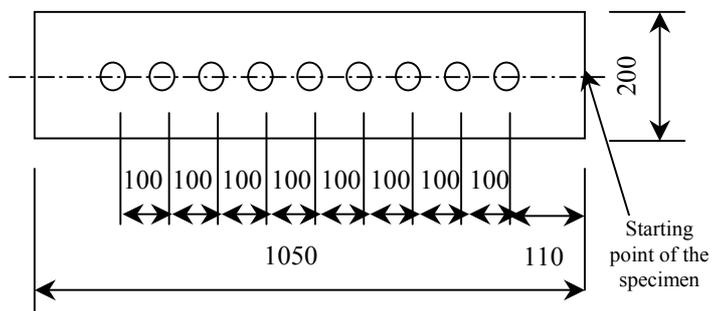
**Fig. 5.** Calibration slab with apertures for heat flux density measurement
