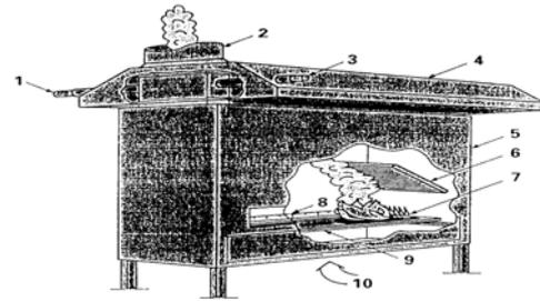
**Fig. 4.** Basic scheme of the equipment: 1, 3 – aperture (if projected); 2 – vent pipe; 4 – vent hood; 5 – test chamber; 6 – the screen surface of heat flux radiation; 7 – flame controlling burner; 8 – scale; 9 – specimen holder with the specimen; 10 – environment air suction through the bottom of the chamber
