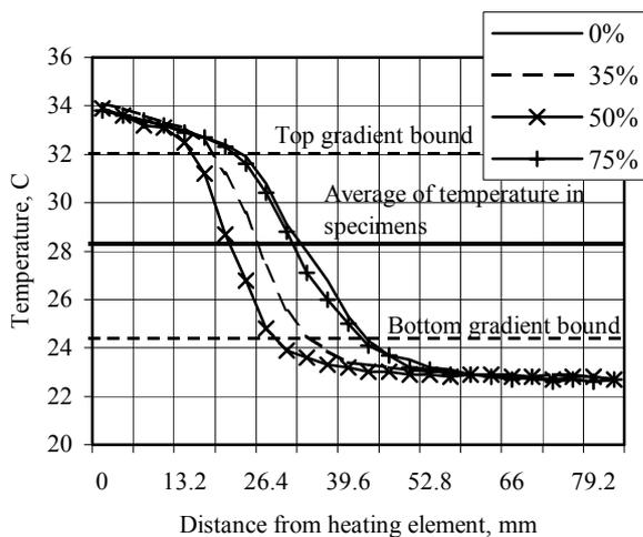
**Fig. 6.** Temperature distribution in specimens with different percentage of damage after heating
