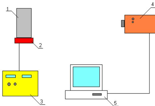
**Fig. 3.** Schematic illustration of the experimental apparatus for the temperature variation detection using infrared spectrum's analysis: 1 – specimen; 2 – heating element; 3 – powers supply; 4 – IR camera; 5 – computer
