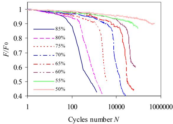
**Fig. 7.** Evolution of the load  $F/F_0$  of hybrid HFRP laminates according the number of  $N$  cycles
