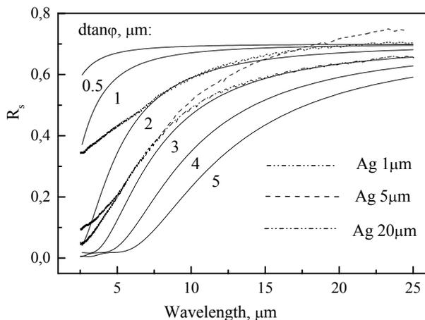
**Fig. 6.** Comparison of experimental (broken curves) and modelled (solid curves) specular reflectance spectra of silver electrodeposits on velour copper
