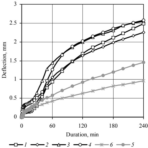
**Fig. 5.** The hardening temperature and tempering duration influence on deflection of steel 95X18 specimens. Tempering temperature 520 °C; normal bending stresses 188 MPa: 1 – 950 °C; 2 – 1000 °C; 3 – 1050 °C; 4 – 1100 °C; 5 – 950 °C, 560 °C × 1 h × 3 times; 6 – 1100 °C, 560 °C × 1 h × 3 times
