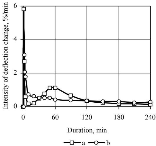
**Fig. 6.** Intensity of deflection of steel 95X18 specimens, hardened from 1100 °C and bended during tempering at 520 °C temperature for 4 hours: a – tempered for the first time after hardening; b – tempered without load at 560 °C temperature 4 times by 1 hour
