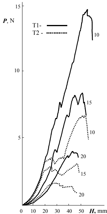
Fig. 2. The curves of specimens T1 and T2 pulling through a rounded hole at h = 5 mm and r = 10 ; 15 and 20 mm
