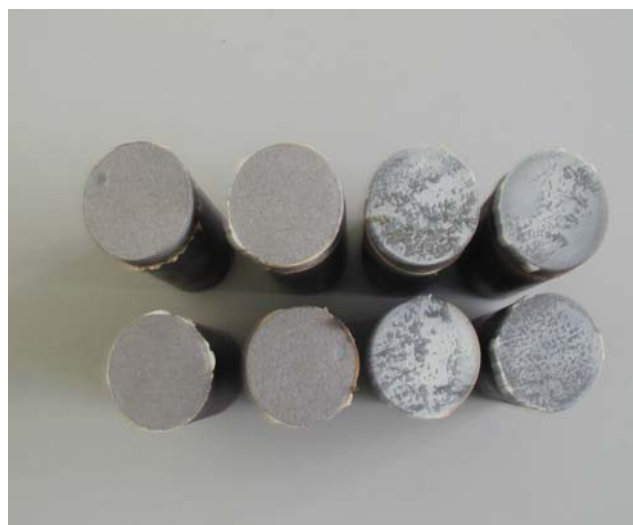
Fig. 3. The samples after bond tensile test (in left rupture occurred in the coating, in right occurred in the glue)
