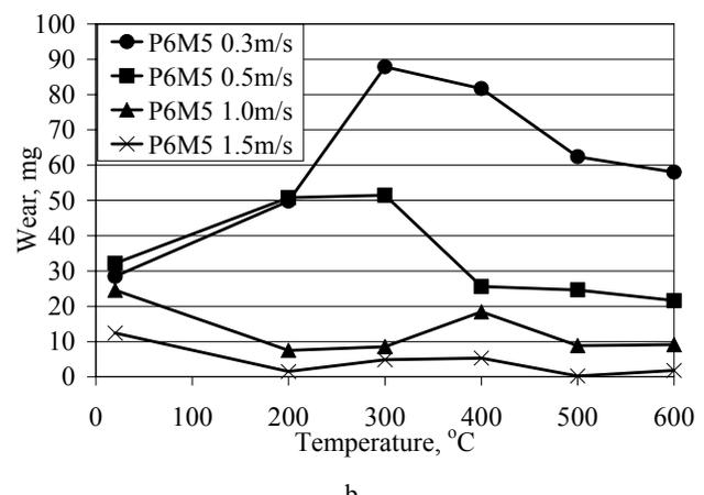
**Fig. 3.** Temperature influence on the wear rate of rotating specimen in pair with couterfase (steel 45) when sliding distance was 2000 m. Rotating specimen: a – WC – 12 % Co coating; b – high speed steel P6M5
