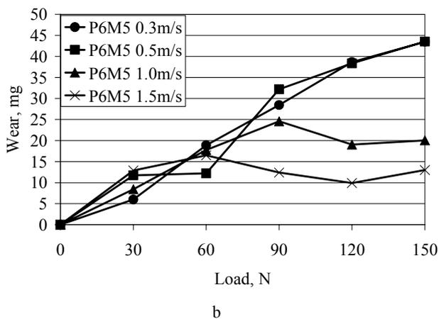
**Fig. 2.** Load influence on the wear rate of rotating specimen in pair with couterfase (steel 45) when temperature is 20°C and sliding distance was 2000 m. Rotating specimen: a – WC – 12 % Co coating; b – high speed steel P6M5
