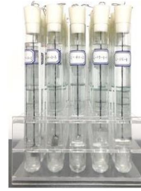
Fig. 2. Immersion specimens in a glass container covered with silicone plug
