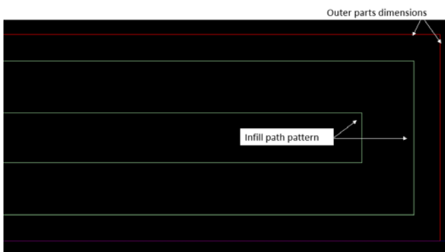
Fig. 2. Raw infill pattern view from the top
