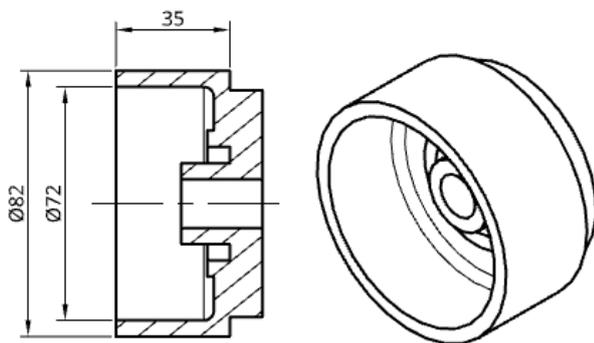
**Fig. 5.** Drawing of Fe–C–Cu PM part
