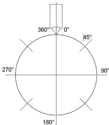
Fig. 9. Illustrates a surface roughness measurement scheme on a circumference of Fe--C -Cu PM part
