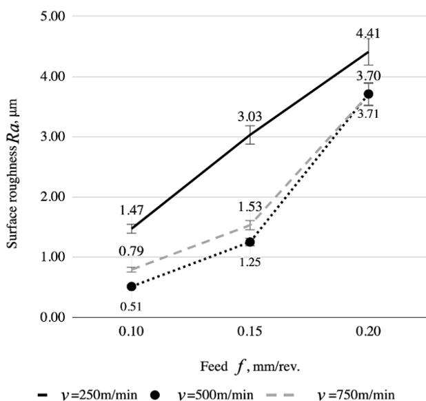
**Fig. 7.** Change of surface roughness  $Ra$  depending on feed under defined steps of the cutting speed ( $v$ )
