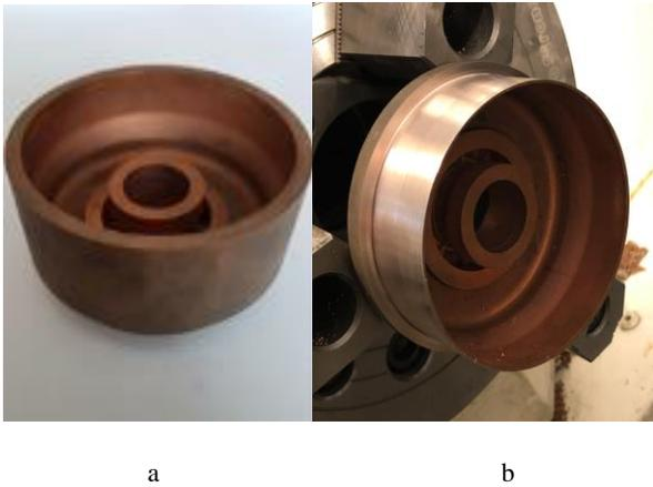
**Fig. 4.** a – Fe–C–Cu PM part to be machined; b – machined Fe–C–Cu PM part in the chuck of the lathe
