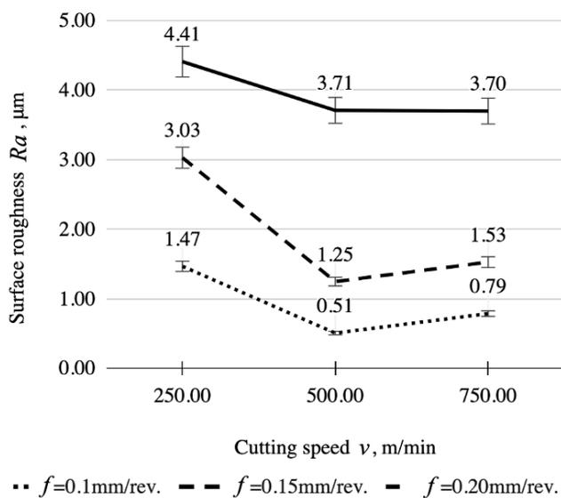
**Fig. 6.** Variation of surface roughness  $Ra$  depending on cutting speed ( $v$ ) under defined steps of the feed ( $f$ )
