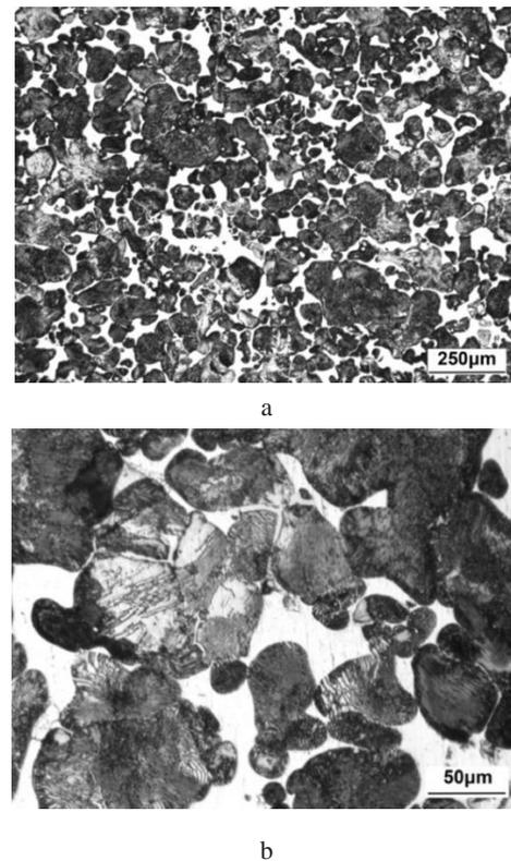
**Fig. 2.** A microstructure of an etched Fe-C -Cu PM part at: a – magnification of 50<sup>x</sup>; b – magnification of 500<sup>x</sup>
