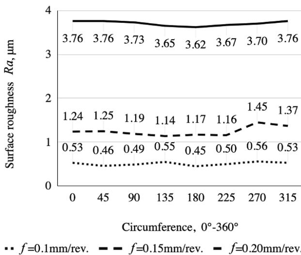
Fig. 8. Distribution of surface roughness on the circumference of the machined cylindrical surface
