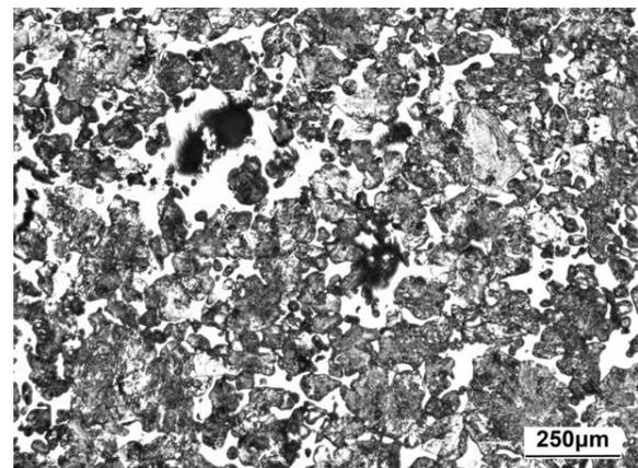
**Fig. 3.** A microstructure of an etched Fe-C -Cu PM part at a magnification of 100<sup>x</sup>
