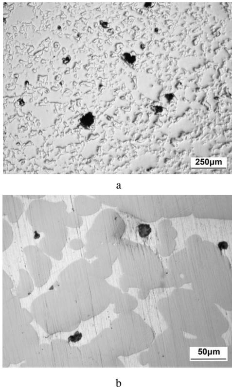
**Fig. 1.** A microstructure of a non-etched Fe-C -Cu PM part at: a – magnification of 50<sup>x</sup>; b – magnification of 500<sup>x</sup>
