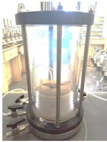
Fig. 2. The reformatory flexible wall permeameter
