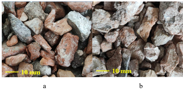
Fig. 4. Apparent phenomenon of BA: a – nano-SiO 2 ; b – nano-Al 2 O 3
