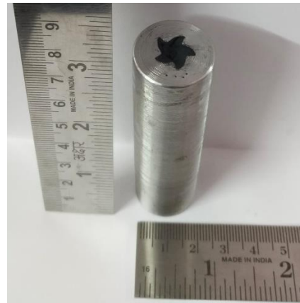
Fig. 3. Infill of MWCNT particles in the female socket of SS316L
