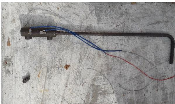
**Fig. 5.** Grouted coupler with connecting rod
