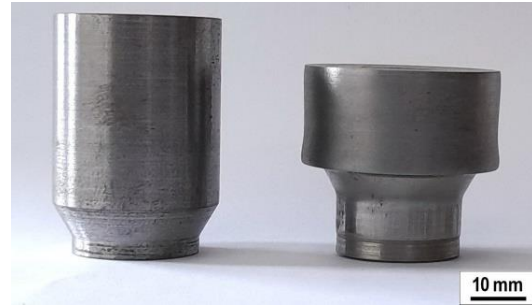
Fig. 2. The starting billet and the extruded element
