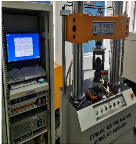
Fig. 4. Fatigue test machine for magnetorheological mounting
