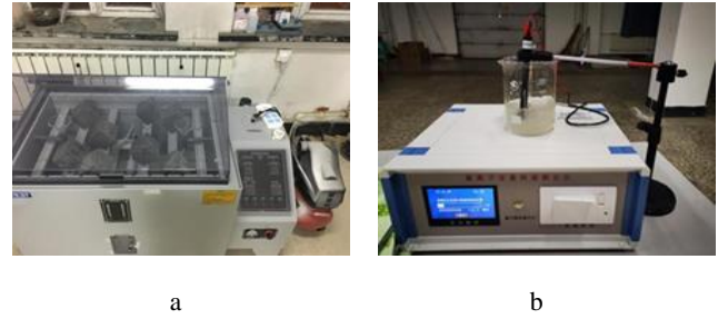
Fig. 1. Experimental equipment: a–KW-ST-90 salt spray test chamber; b–JY-20 quick measuring instrument
