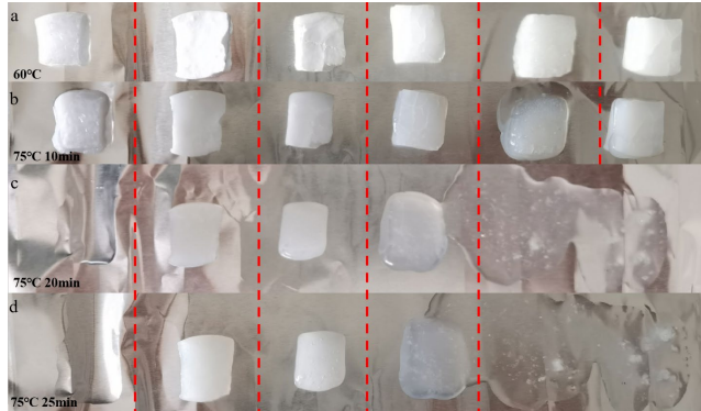
Fig. 10. Digital photographs obtained by placing PEG and CNPCMs in the oven at 60 °C and 75 °C (PEG, CNPCM1, CNPCM2, CNPCM3, CNPCM4, and CNPCM5 from left to right)
