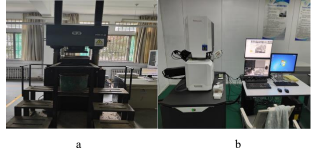
Fig. 1. Test equipment: a – servo-hydraulic machine; b – scanning electron microscope
