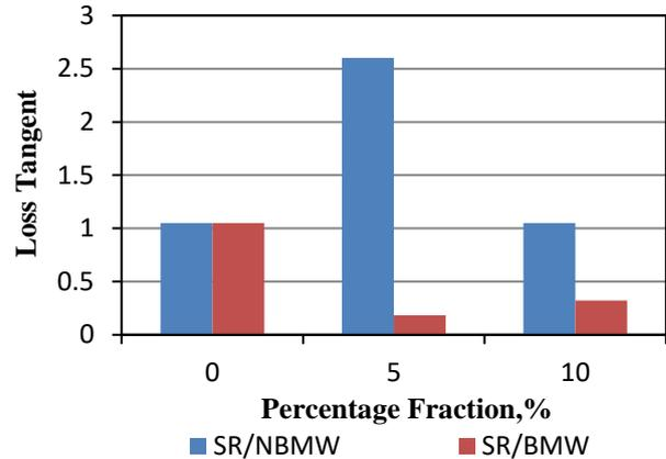
**Fig. 13.** The loss tangent calculated in the frequency range of 7–7.98 GHz for  $\text{Na}_{0.5}\text{Bi}_{0.5}\text{Mo}_{0.5}\text{W}_{0.5}\text{O}_4$ /silicone rubber composite, and  $\text{Bi}_2\text{Mo}_{0.5}\text{W}_{0.5}\text{O}_6$ /silicone rubber composite as a function of volume fraction of fillers
