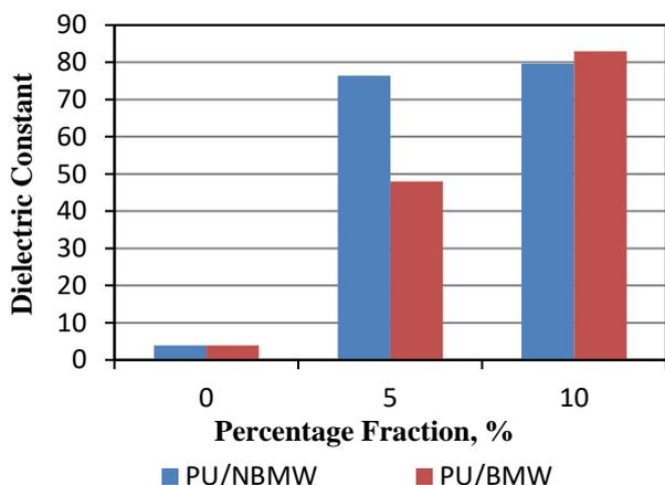
**Fig. 6.** The dielectric constant calculated in the frequency range of 7–7.98 GHz for  $\text{Na}_{0.5}\text{Bi}_{0.5}\text{Mo}_{0.5}\text{W}_{0.5}\text{O}_4$ /polyurethane composite, and  $\text{Bi}_2\text{Mo}_{0.5}\text{W}_{0.5}\text{O}_6$ /polyurethane composite as a function of volume fraction of fillers
