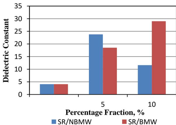
**Fig. 7.** The dielectric constant calculated in the frequency range of 7–7.98 GHz for  $\text{Na}_{0.5}\text{Bi}_{0.5}\text{Mo}_{0.5}\text{W}_{0.5}\text{O}_4$ /silicone rubber composite, and  $\text{Bi}_2\text{Mo}_{0.5}\text{W}_{0.5}\text{O}_6$ /silicone rubber composite as a function of volume fraction of fillers
