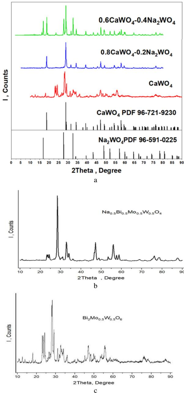
**Fig. 1.** a – the X-ray diffraction patterns of  $(1-x)\text{CaWO}_4-x\text{Na}_2\text{WO}_4$  ( $x = 0, 0.2, 0.4$ ) ceramics; b – the XRD pattern of  $\text{Na}_{0.5}\text{Bi}_{0.5}\text{Mo}_{0.5}\text{W}_{0.5}\text{O}_4$  ceramic; c – the XRD pattern of  $\text{Bi}_2\text{W}_{0.5}\text{Mo}_{0.5}\text{O}_6$  ceramic
