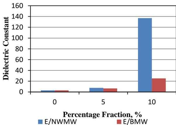
**Fig. 5.** The dielectric constant calculated in the frequency range of 7–7.98 GHz for  $\text{Na}_{0.5}\text{Bi}_{0.5}\text{Mo}_{0.5}\text{W}_{0.5}\text{O}_4$ /epoxy composite, and  $\text{Bi}_2\text{Mo}_{0.5}\text{W}_{0.5}\text{O}_6$ /epoxy composite as a function of volume fraction of fillers
