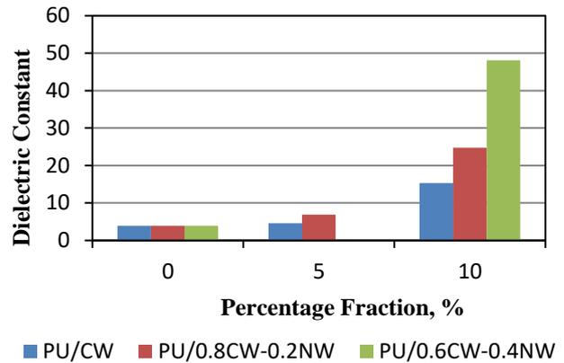
**Fig. 3.** The dielectric constant calculated in the frequency range of 7–7.98 GHz for  $\text{CaWO}_4$ /polyurethane composite,  $0.8\text{CaWO}_4\text{-}0.2\text{Na}_2\text{WO}_4$  /polyurethane composite and  $0.6\text{CaWO}_4\text{-}0.4\text{Na}_2\text{WO}_4$ /polyurethane composite as a function of volume fraction of fillers
