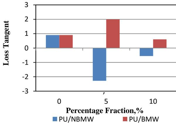
**Fig. 12.** The loss tangent calculated in the frequency range of 7–7.98 GHz for  $\text{Na}_{0.5}\text{Bi}_{0.5}\text{Mo}_{0.5}\text{W}_{0.5}\text{O}_4$ /polyurethane composite, and  $\text{Bi}_2\text{Mo}_{0.5}\text{W}_{0.5}\text{O}_6$ /polyurethane composite as a function of volume fraction of fillers
