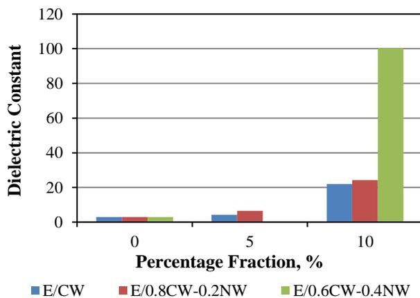
**Fig. 2.** The dielectric constant calculated in the frequency range of 7–7.98 GHz for  $\text{CaWO}_4$ /epoxy composite,  $0.8\text{CaWO}_4\text{-}0.2\text{Na}_2\text{WO}_4$  /epoxy composite and  $0.6\text{CaWO}_4\text{-}0.4\text{Na}_2\text{WO}_4$ /epoxy composite as a function of volume fraction of fillers
