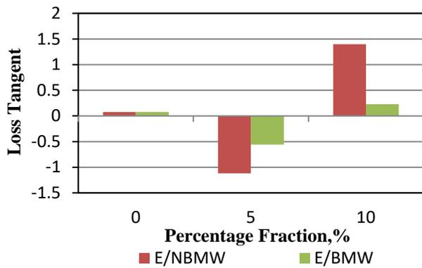
**Fig. 11.** The loss tangent calculated in the frequency range of 7–7.98 GHz for  $\text{Na}_{0.5}\text{Bi}_{0.5}\text{Mo}_{0.5}\text{W}_{0.5}\text{O}_4$ /epoxy composite, and  $\text{Bi}_2\text{Mo}_{0.5}\text{W}_{0.5}\text{O}_6$ /epoxy composite as a function of volume fraction of fillers
