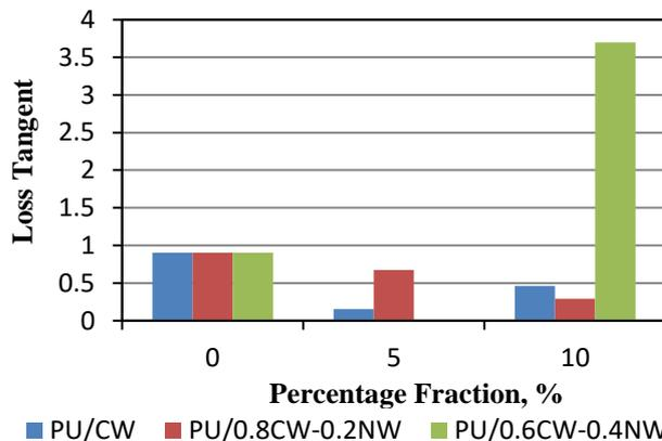
**Fig. 9.** The loss tangent calculated in the frequency range of 7–7.98 GHz for  $\text{CaWO}_4$ /polyurethane composite,  $0.8\text{CaWO}_4-0.2\text{Na}_2\text{WO}_4$ /polyurethane composite and  $0.6\text{CaWO}_4-0.4\text{Na}_2\text{WO}_4$ /polyurethane composite as a function of volume fraction of fillers
