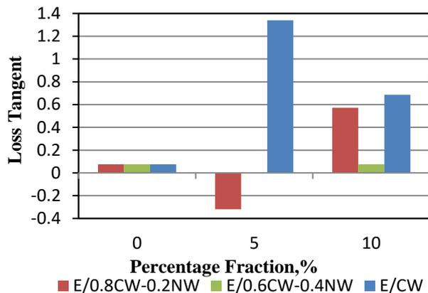
**Fig. 8.** The loss tangent calculated in the frequency range of 7–7.98 GHz for  $\text{CaWO}_4$ /epoxy composite,  $0.8\text{CaWO}_4-0.2\text{Na}_2\text{WO}_4$ /epoxy composite and  $0.6\text{CaWO}_4-0.4\text{Na}_2\text{WO}_4$ /epoxy composite as a function of volume fraction of fillers
