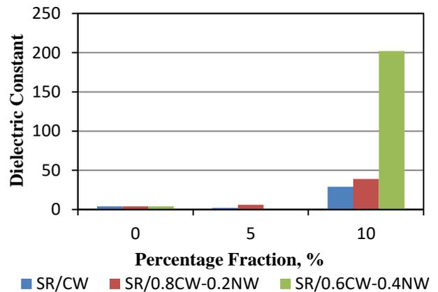
**Fig. 4.** The dielectric constant calculated in the frequency range of 7–7.98 GHz for  $\text{CaWO}_4$ /silicone rubber composite,  $0.8\text{CaWO}_4\text{-}0.2\text{Na}_2\text{WO}_4$  /silicone rubber composite and  $0.6\text{CaWO}_4\text{-}0.4\text{Na}_2\text{WO}_4$ /silicone rubber composite as a function of volume fraction of fillers
