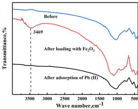
**Fig. 22.** FTIR patterns of geopolymer porous ceramic samples before and after loading with  $\text{Fe}_2\text{O}_3$  and  $\text{Fe}_2\text{O}_3/\text{geopolymer}$  porous ceramic samples after adsorption of  $\text{Pb}(\text{II})$
