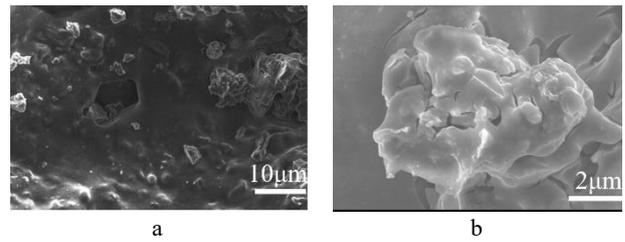
**Fig. 8.** SEM images of  $\text{Fe}_2\text{O}_3$ /geopolymer porous ceramic samples prepared by calcining at  $450^\circ\text{C}$  for 6 hours: a— $\times 1000$  magnification; b— $\times 5000$  magnification
