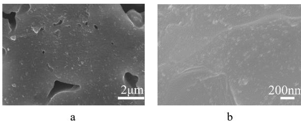
**Fig. 7.** SEM images of  $\text{Fe}_2\text{O}_3$ /geopolymer porous ceramic samples prepared by calcining at  $450^\circ\text{C}$  for 1 hour: a— $\times 5000$  magnification; b— $\times 50000$  magnification
