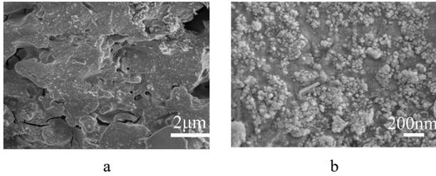
**Fig. 5.** SEM images of  $\text{Fe}_2\text{O}_3$ /geopolymer porous ceramic samples prepared by calcining at  $450^\circ\text{C}$  for 2 hours: a— $\times 5000$  magnification; b— $\times 50000$  magnification
