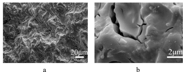
**Fig. 11.** SEM images of  $\text{Fe}_2\text{O}_3$ /geopolymer porous ceramic samples prepared by impregnating in 0.6M  $\text{Fe}(\text{NO}_3)_3$ : a— $\times 1000$  magnification; b— $\times 5000$  magnification
