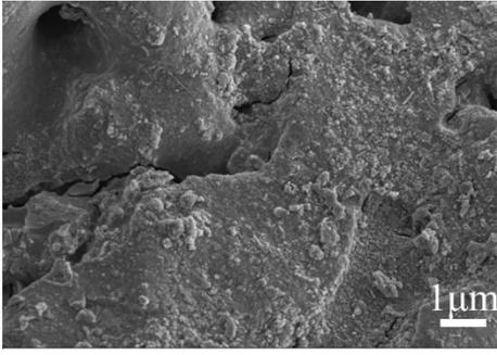
**Fig. 20.** SEM images of  $\text{Fe}_2\text{O}_3/\text{geopolymer}$  porous ceramic samples after adsorption of  $\text{Pb}(\text{II})$
