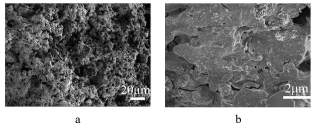
**Fig. 10.** SEM images of  $\text{Fe}_2\text{O}_3$ /geopolymer porous ceramic samples prepared by impregnating in 0.2M  $\text{Fe}(\text{NO}_3)_3$ : a— $\times 1000$  magnification; b— $\times 5000$  magnification
