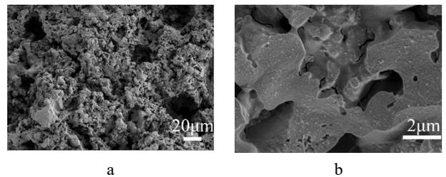
**Fig. 9.** SEM images of  $\text{Fe}_2\text{O}_3$ /geopolymer porous ceramic samples prepared by impregnating in 0.1M  $\text{Fe}(\text{NO}_3)_3$ : a— $\times 1000$  magnification; b— $\times 5000$  magnification
