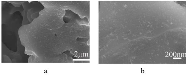
**Fig. 4.** SEM images of  $\text{Fe}_2\text{O}_3$ /geopolymer porous ceramic samples prepared by calcining at  $350^\circ\text{C}$  for 2 hours: a— $\times 5000$  magnification; b— $\times 50000$  magnification
