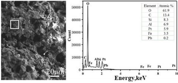
**Fig. 21.** SEM-EDS images of  $\text{Fe}_2\text{O}_3/\text{geopolymer}$  porous ceramic samples after adsorption of  $\text{Pb}(\text{II})$
