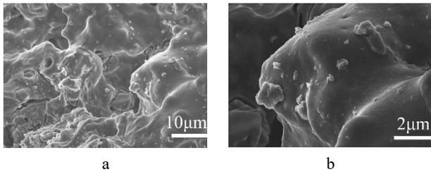
**Fig. 6.** SEM images of  $\text{Fe}_2\text{O}_3$ /geopolymer porous ceramic samples prepared by calcining at  $650^\circ\text{C}$  for 2 hours: a— $\times 1000$  magnification; b— $\times 5000$  magnification
