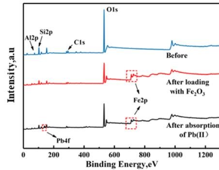
**Fig. 23.** Survey XPS pattern of geopolymer porous ceramic samples before and after loading with  $\text{Fe}_2\text{O}_3$  and  $\text{Fe}_2\text{O}_3/\text{geopolymer}$  porous ceramic samples after adsorption of  $\text{Pb}(\text{II})$
