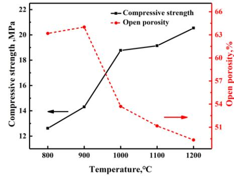
Fig. 2. Effects of sintering temperature on physical properties of geopolymer porous ceramic samples
