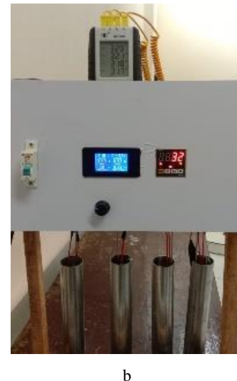
Fig. 1. The apparatus for operation evaluation of LHSM as LTES: a – schematic; b – photograph
