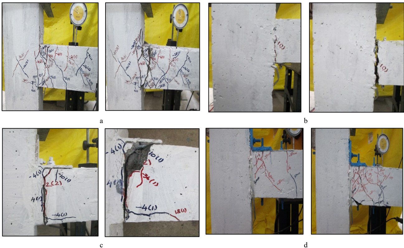
Fig. 9. Crack pattern of the monolithic and precast specimens: a – monolithic Specimen; b – billet with dowel; c – billet with dowel-cleat angle; d – extended billet dowel-cleat angle
