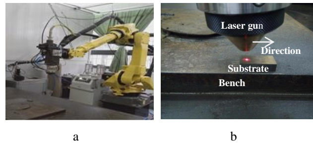
Fig. 1. a–laser cladding equipment used in this test; b–a schematic picture of the laser cladding process
