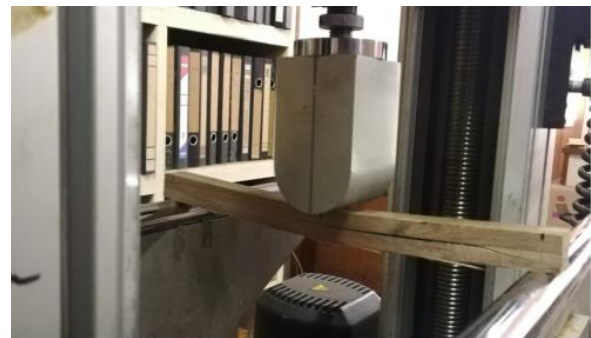
Fig. 4. Static bending testing
