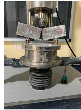
Fig. 6. Flexural tensile strength test
