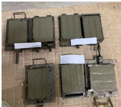
Fig. 4. Samples casting for (4 \times 4 \times 16) \text{ cm}^3 specimens
