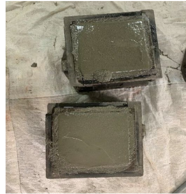
Fig. 7. samples casting for (15 \times 15 \times 15) \text{ cm}^3 specimens
