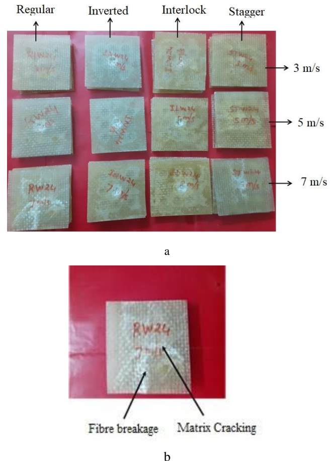
Fig. 5. a–top damage portion of the SCSS; b–typical photograph of the top side of R at 7 m/s impact velocity
