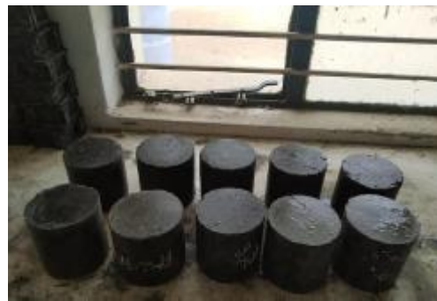
Fig. 9. Specimen for sorptivity test
