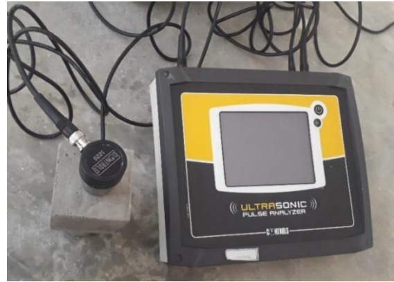
Fig. 8. Apparatus used for ultrasonic pulse velocity
