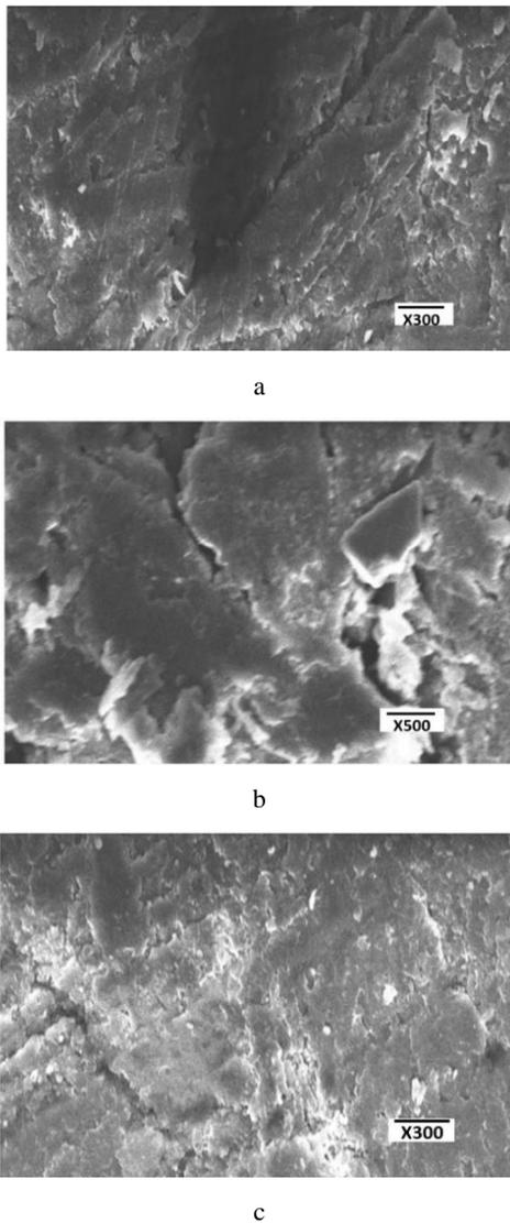
**Fig. 6.** SEM images of the tensile fracture surface of composite exposed to the groundwater environment
