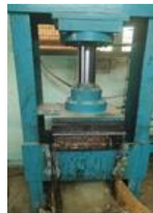
Fig. 2. Digital image of hot press compression moulding machine [21]
