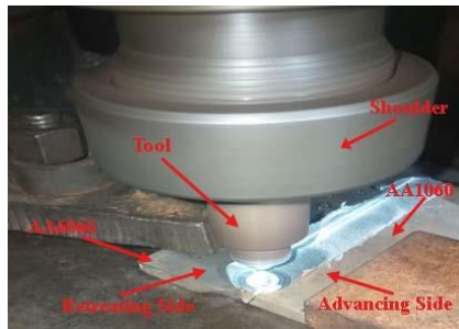
Fig. 1 FSW processes for the alloys AA6066-T6 and AA1060-T6
