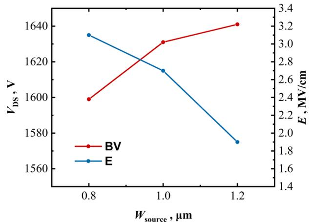
Fig. 5. The effect of  $w_{\text{source}}$  change from  $0.8 \mu\text{m}$  to  $1.2 \mu\text{m}$  on the breakdown characteristics of the device
