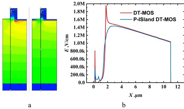
**Fig. 11.** p-island DT-MOS and DT-MOS at 1200 V: a–electric field intensity distribution; b–absolute value of electric field intensity along the cutting line through the gate oxide layer
