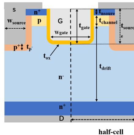
**Fig. 1.** Structure cross-section of DT-MOS device
