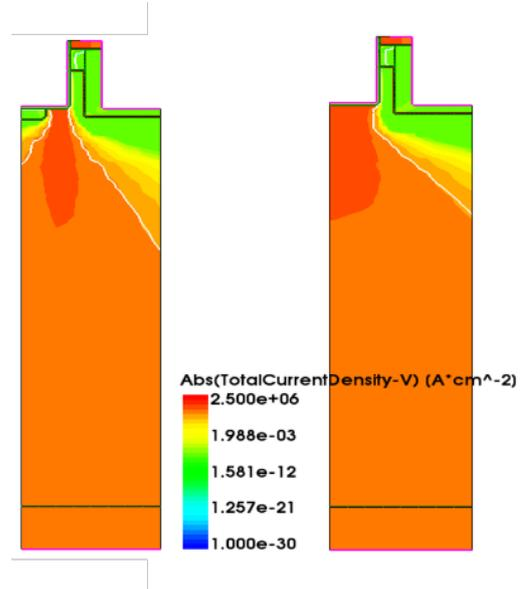
Fig. 10. Current density distribution of p-island DT-MOS and DT-MOS at  $V_{GS} = 10 \text{ V}$  and  $V_{DS} = 50 \text{ V}$
