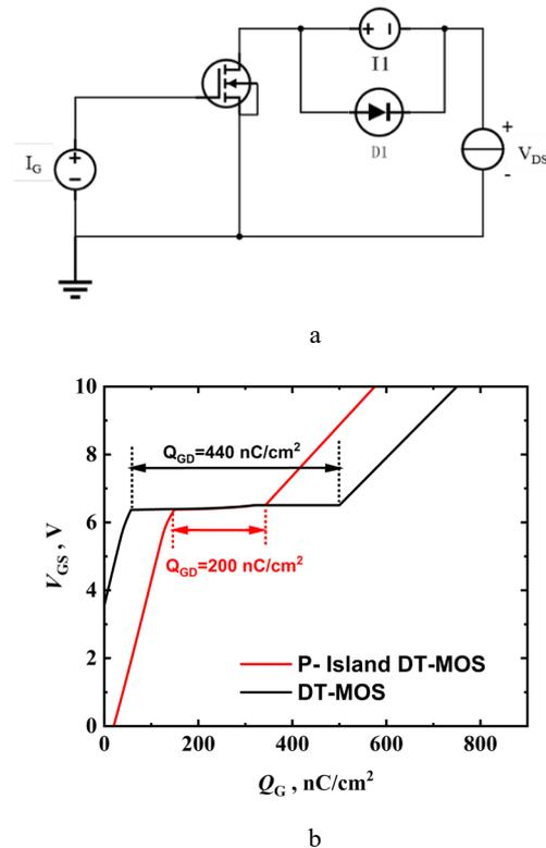
**Fig. 13.** a–gate charge test circuit; b–comparison of gate charge waveforms of p-island DT-MOS and DT-MOS
