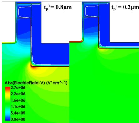
Fig. 3. The change of electric field strength when  $t_{p^+}$  changes from  $0.2 \mu\text{m}$  to  $0.8 \mu\text{m}$
