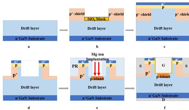
**Fig. 14.** Potential process manufacturing flow for p-island DT-MOS including MOCVD selection epitaxy and ion implantation
