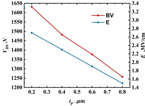
Fig. 2. The effect of  $t_{p^+}$  change from  $0.2 \mu\text{m}$  to  $0.8 \mu\text{m}$  on the breakdown characteristics of the device
